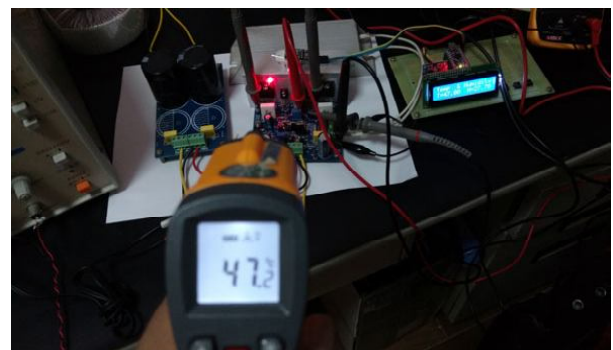
Temperature manual check using Infrared Temperature sensor
