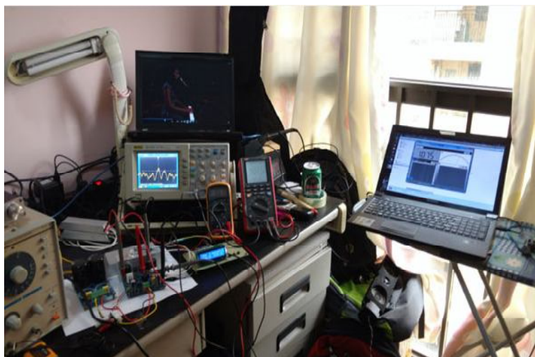
Temperature monitoring the heatsink using customized programmed Arduino hardware
