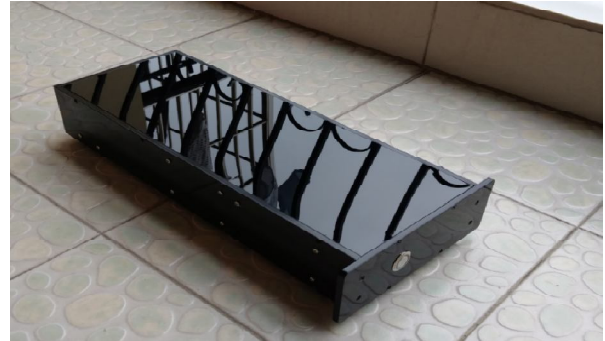
Final fiber glass casing - a fully working DNY40W power amplifier project
